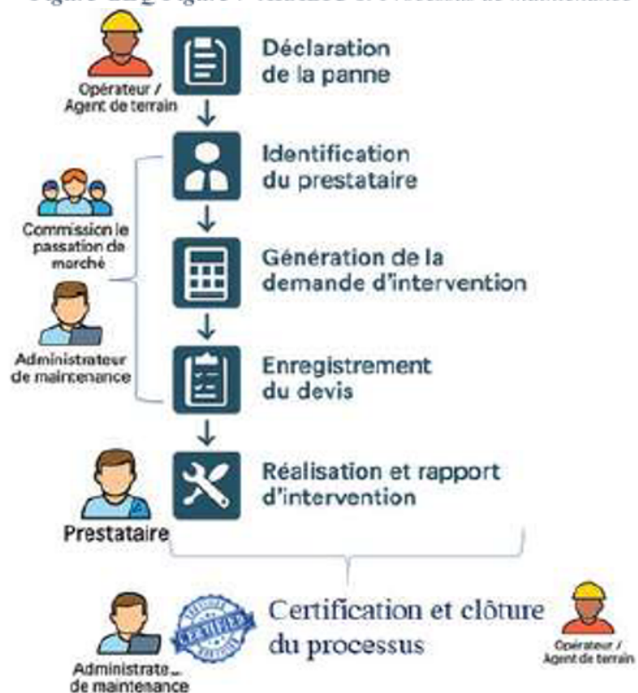
Figure SEQ Figure \* ARABIC 6: Processus de maintenance
